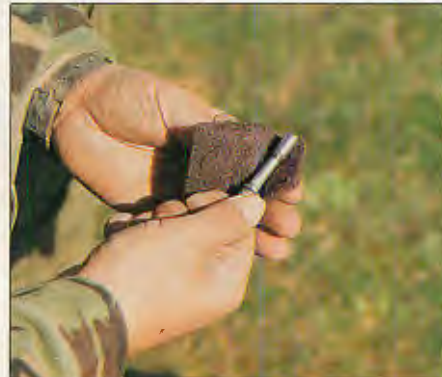
9 Carbon fouling is cleaned off the bolt with a nylon pad. With a little oil this will also remove rust but, like a pan scourer, should not be used on weapon parts coated with a protective finish.
